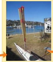
Then move the retractable dog lead switch to 'retract' and pull the boom down into the sailing position by means of the mainsheet. Switch RDL back to 'stop'. Sail away.
